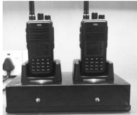
Figure 8 - Two-way battery charger for Creeper DMR
