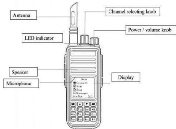
Figure 11 - Main Parts of the Creeper DMR
